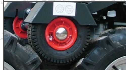
Carrier wheel disengages for easy wheel changing
