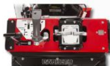
Easy controls operate the track drive and cutter wheel
