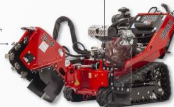
Sixteen T00 series carbide Greenteeth® with three cutting surfaces
